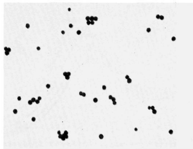
Fig. 1.—Electron micrograph of gold hydrosol, S-1 (sodium citrate). Magnification: 80,000 diameters, 1 mm. = 125 Å.
